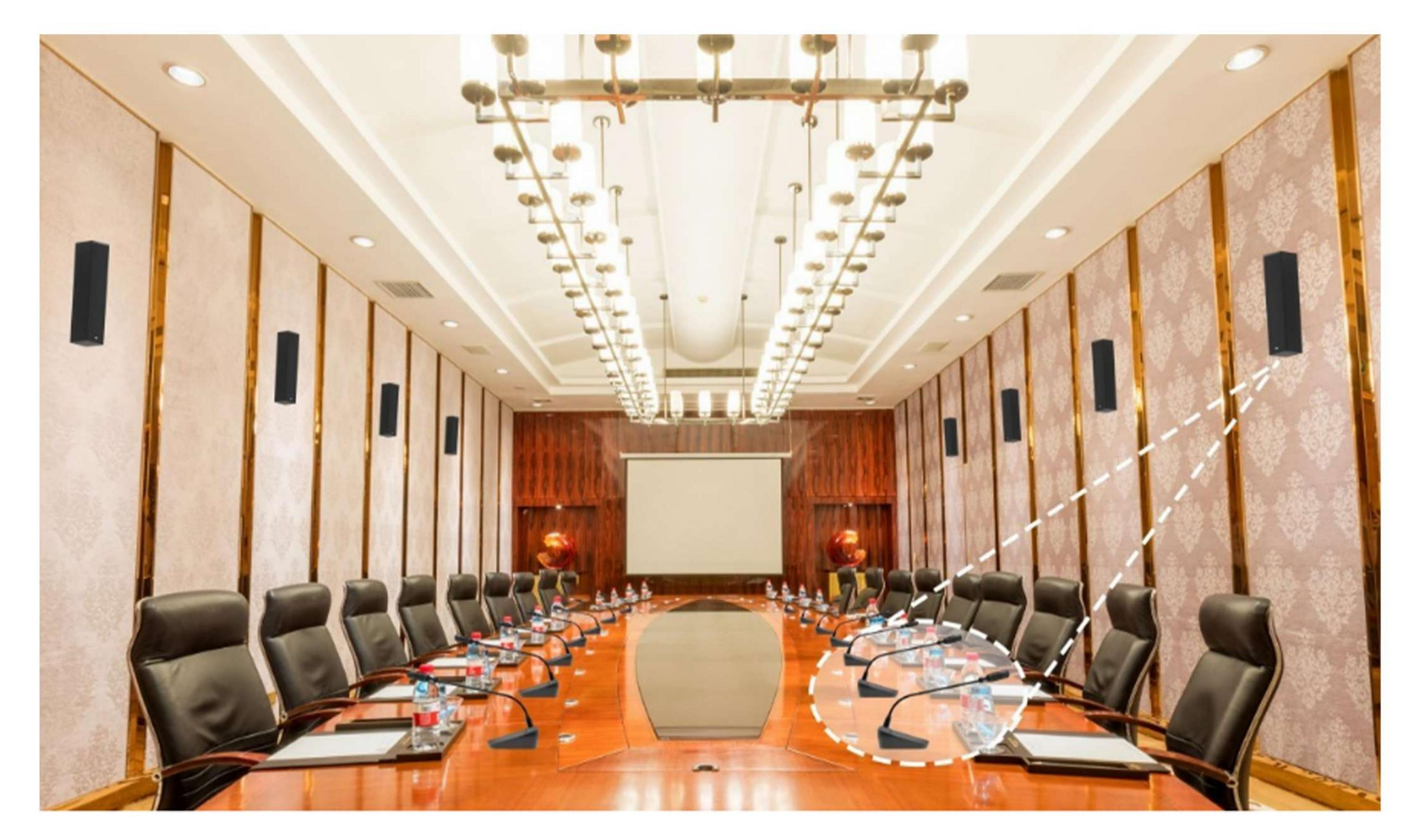
Mix Minus Technology: After setting the zone phase control function, it can intelligently recognize the current using microphones and control the volume of the nearby speakers, to solve the howling problem.
